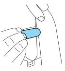
The end of the shoulder belt **must** be clipped in order to keep it from striking anything during vehicle operation.
